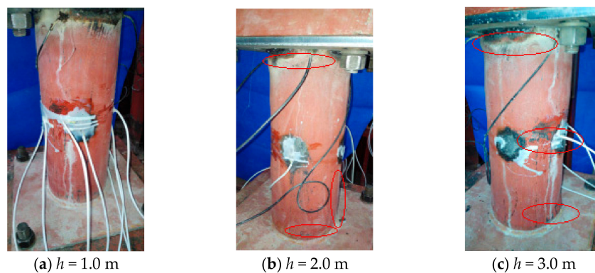
Figure 12. The failure mode of CFST with 3 mm wall thickness.
