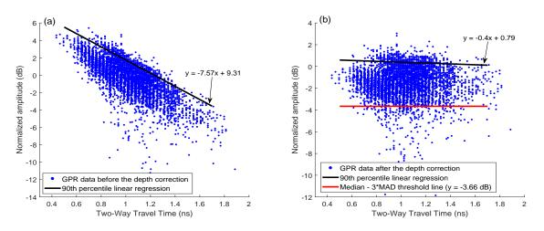
**Figure 13.** Scatter plot of GPR data points from the curved bridge (**a**) before and (**b**) after amplitudedepth correction, and threshold line.
