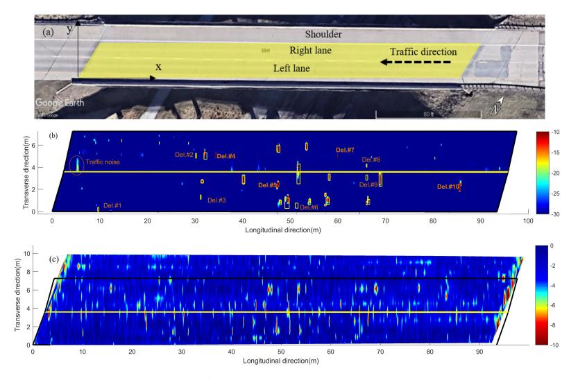
Figure 8. Straight concrete bridge deck: (a) Google Earth image; (b) acoustic scanning image; (c) GPR attenuation image.
