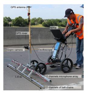
Figure 1. 12-channel acoustic scanning cart.
