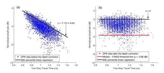
**Figure 6.** Scatter plot of GPR data points (**a**) before and (**b**) after amplitude-depth correction and 90th percentile linear regression from the bridge with sound concrete.
