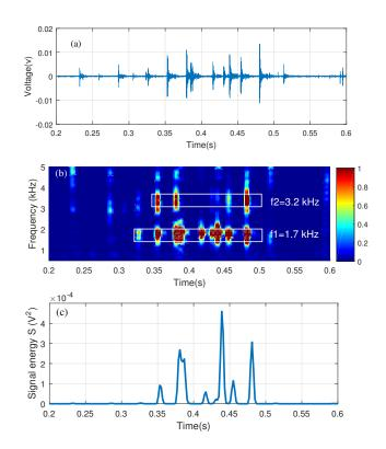
**Figure 2.** Ball-chain test results: (**a**) time-domain signal; (**b**) STFT spectrogram with normalized amplitude; (**c**) signal energy.
