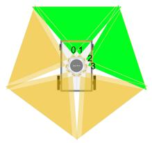
**Figure A2.** Pentagonal camera rig mounted on the robot (left). The first four cameras were included in the challenge data (right), green colour indicates their fields of view.
