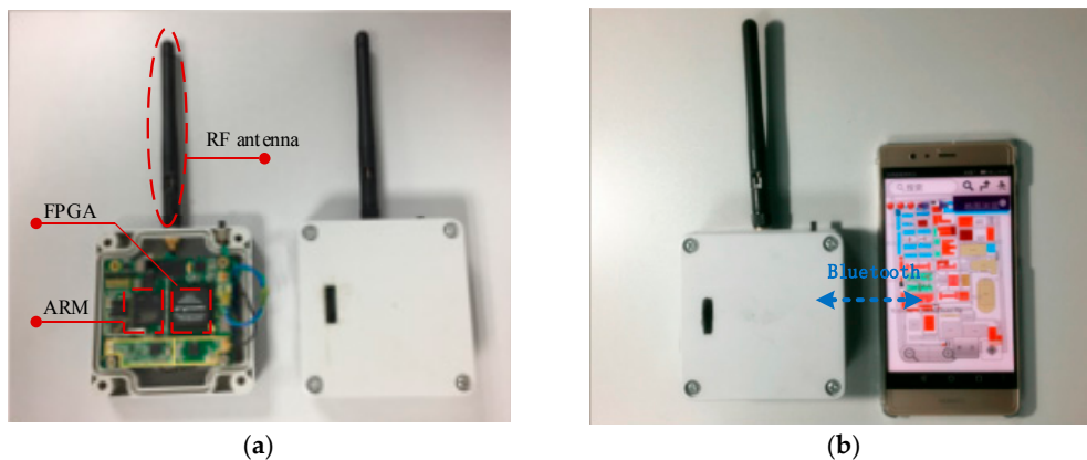
Figure 13. The TC-OFDM receiver. (a) is the internal and external structure of the TC-OFDM receiver; and (b) is the communication between the positioning receiver and the mobile phone.
