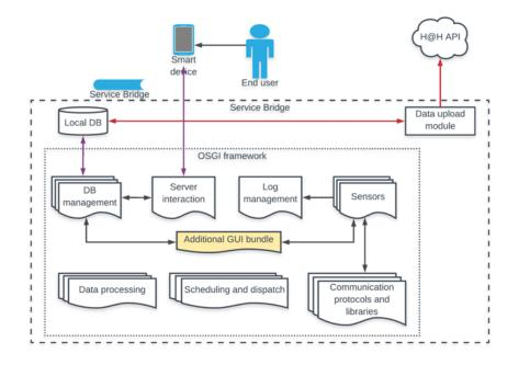
Figure 3. Concept of the Smart Home architecture developed and tested in the pilot case.
