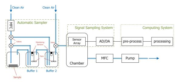
Figure 3. Gas/odor concentration measurement system with an automatic sampler.
