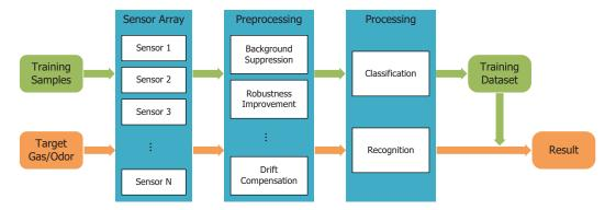
Figure 2. A typical scheme of machine olfaction.
