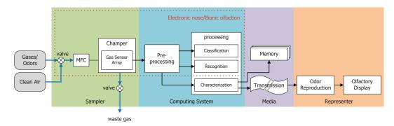
Figure 1. A typical scheme of machine olfaction. MFC, mass flow control.
