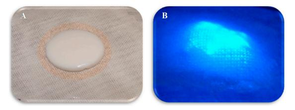
**Figure 6.** Depiction of pNA conjugate biosensor with protease activation that is interfaced in a multilayer bandage prototype both with and without ultraviolet activation [52]. Image (**A**,**B**): demonstrates the gauze contact layer and the aerogel biosensor layer with and without ultraviolet.
