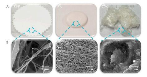
**Figure 1.** Images of the cellulosic (CFP, blue) and nanocellulosic (NA, pink and NC, green) transducers as (**A**) optical and (**B**) FE-SEM images.
