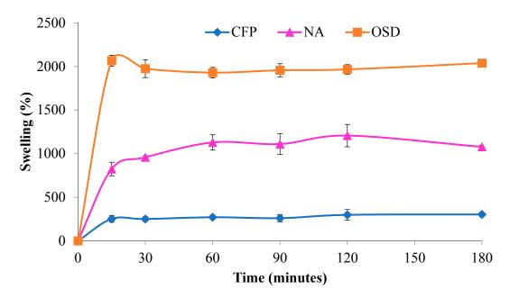
**Figure 3.** Moisture absorption (Millipore water) of cellulosic filter paper (blue), nanocellulosic aerogel (pink), and commercially available sequestrant dressings (orange).
