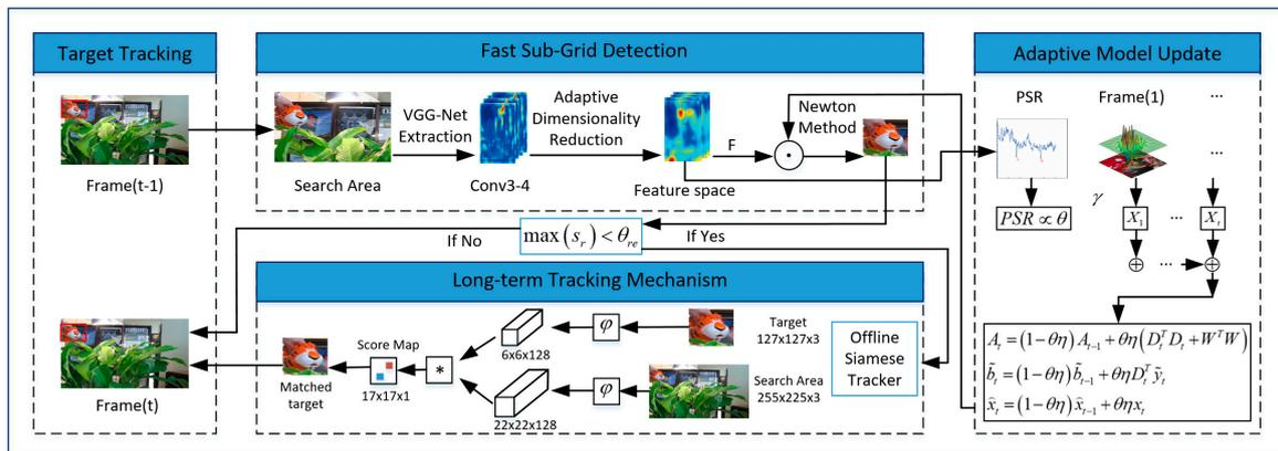
Figure 1. Flow chart of the proposed tracking algorithm.
