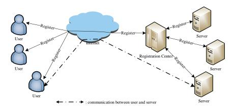
Figure 1. The architecture of the multi-server authentication system.
