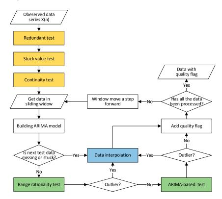
**Figure 2.** The seafloor observatories data quality control operational framework. Orange denotes the general pretest process, green denotes the outlier detection process, and blue denotes the data interpolation process.
