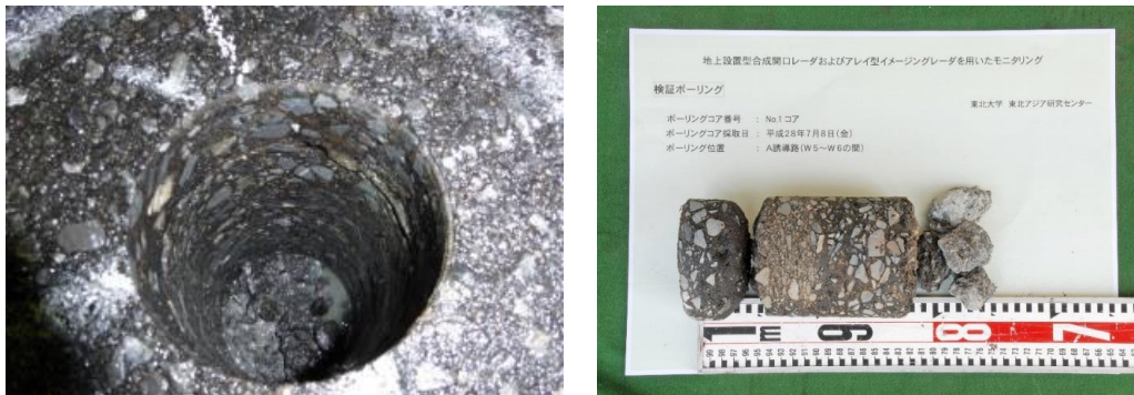
Figure 11. Coring sample acquired from the damaged pavement ( x = 6 m) at the Sendai Airport site.
