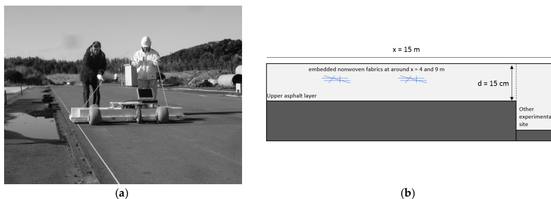
Figure 7. Data acquisition with Yakumo on the airport runway model at the Nobi experiment site. (a) Experiment site. (b) Pavement structure.
