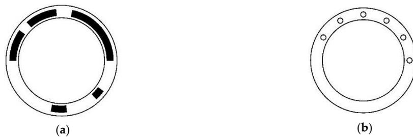
**Figure 4.** Disc pattern and reading head distribution of absolute encoder using a length-6 period-36 necklace ordering STGC. (a) Schematic of the coding disc, where the white area indicates “0”, and the black area indicates “1”; (b) Schematic of the reading disc, where the six small circles denote the six reading heads and are evenly distributed around the half coding track.
