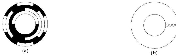
**Figure 1.** Disc pattern and reading head distribution of absolute encoder using a length-4 Gray code: (a) Schematic of the coding disc, where the white area indicates “0”, and the black area indicates “1”; (b) Schematic of the reading disc, where the four small circles denote the four reading heads corresponding to the four coding tracks.
