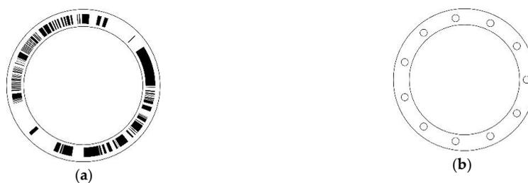
**Figure 2.** Disc pattern and reading head distribution of absolute encoder using a length-11 period-2046 STGC. (a) Schematic of the coding disc, where the white area indicates “0”, and the black area indicates “1”; (b) Schematic of the reading disc, where the 11 small circles denote the 11 reading heads and are evenly distributed around the coding track.
