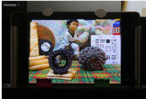
**Figure 8.** The integral image of Figure 7d projected in our 3D InI display prototype.
