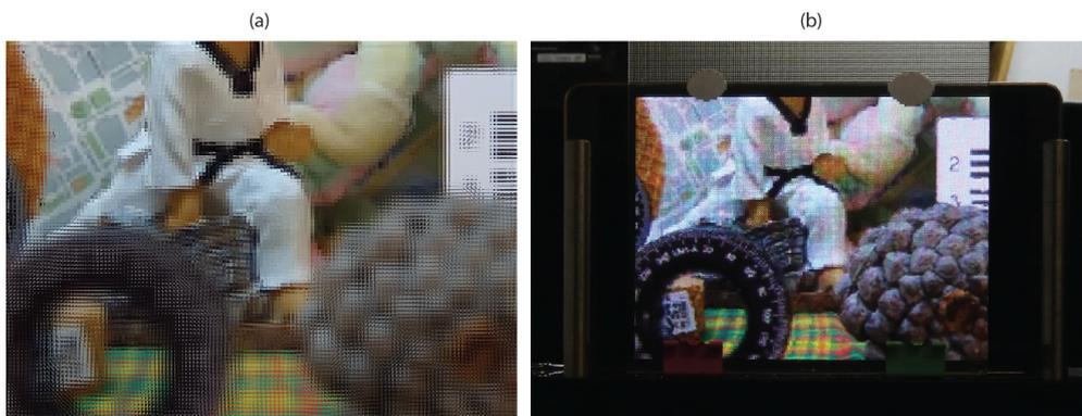
**Figure 9.** Field of view selection: (a) The integral image obtained with the same reference plane and pitch of Figure 7d, with half its field of view ( $z = 2$ ). (b) Projection in 3D InI display.
