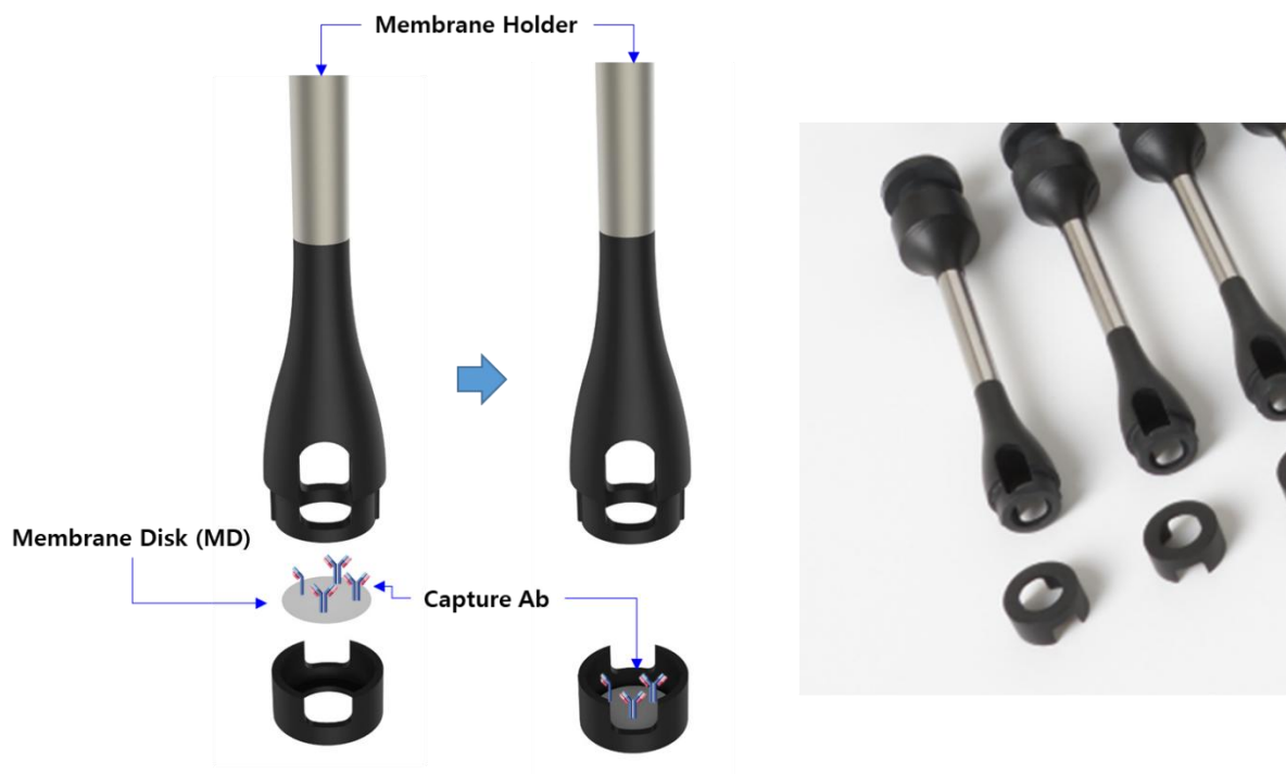
Figure S2. Custom-made membrane disk holder. Capture antibodies were immobilized on the MD and the MD were stationed between holder and its lid.
