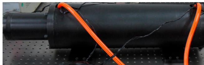
**Figure 10.** Experimental prototype of a giant magnetostrictive actuator.
