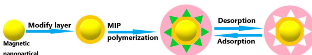
Figure 12. Schematic configuration of the producing process of a magnetic-MIP bioprobe.
