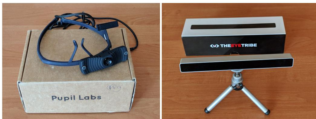
**Figure 6.** Eye trackers used during the experimental part of the research. Left: Pupil Labs headset eye tracker, right: The Eye Tribe remote eye tracker to be mounted below a screen.
