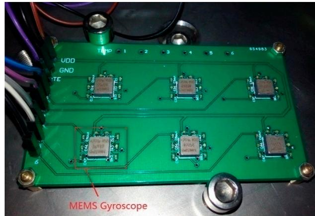
**Figure 4.** Prototype of the gyro array.
