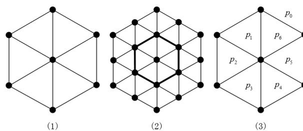
**Figure 1.** Schematics of  $n$ -dimensional hexagonal meshes,  $HX(n)$ : (1)  $HX(2)$ , (2)  $HX(3)$ , and (3) all of the faces in  $HX(2)$ .
