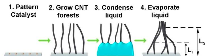
**Figure 3.** Successive steps used in the CNT capillary self-assembly process. Reproduced from [29], courtesy of Michael De Volder.
