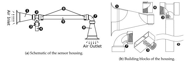
Figure 4. 1 Inlet, 2 Housing-Sensor Holder Coupler, 3 iMet XQ2 Sensor Adapter, 4 iMet XQ2 sensor, 5 Carbon Fiber Tube, 6 Carbon Fiber Tube Adapter, 7 L-bend, and 3 Outlet.
