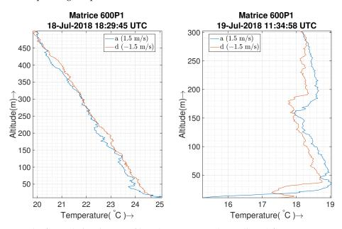
**Figure 14.** The first subplot shows unfiltered temperature data collected from 10 m–500 m of a well-mixed atmosphere at noon with a ground wind of 1.6 m/s with a 5 m/s gust.
