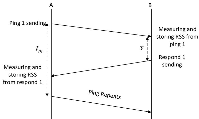
Figure 4. The mechanism of RSS channel characteristics measurement.
