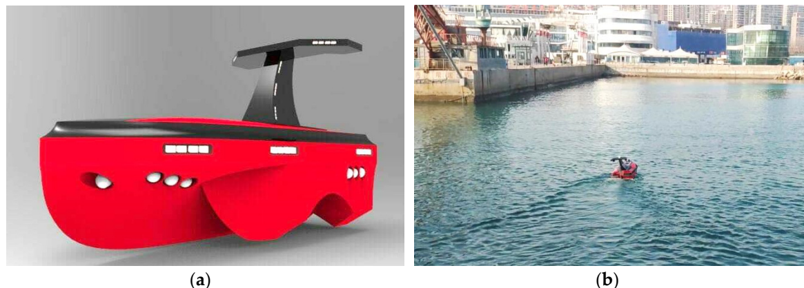
Figure 6. A self-developed unmanned surface vehicle: (a) 3D model; (b) USV in water.
