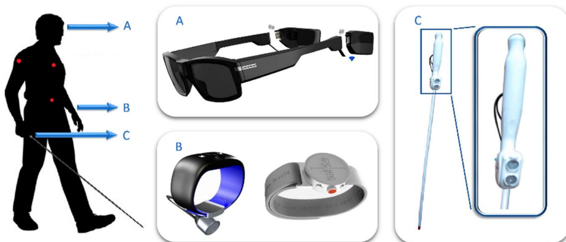
Figure 7. Wearables for the BVI: common placements.
