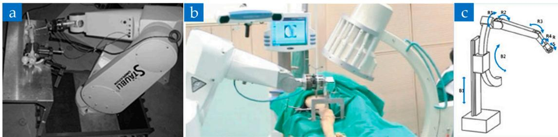
**Figure 2.** Various serial structure orthopedic trauma surgery robot based on an industrial robot. (a) RepoRobo designed by Regensburg Clinical University [48]. (b) Long bone fracture reduction robot system studied by R. Westphal et al. [8]. (c) An orthopedic robot with circular prismatic joint [53].
