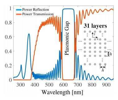
**Figure 1.** Power reflection (blue line) and power transmission (red line) of a 31-layered plasmonic crystal formed by the corresponding periodical arrangement of cylindrical Ag nanocylinders. Period of the grating was equal to h = 300 nm and radius of the nanocylinder amounts to r = 40 nm. Excitation was provided by an impinging H-polarized plane wave ( $H_z$ ,  $E_x$ ,  $E_y$ ) with normal incidence (along the positive y-axis).
