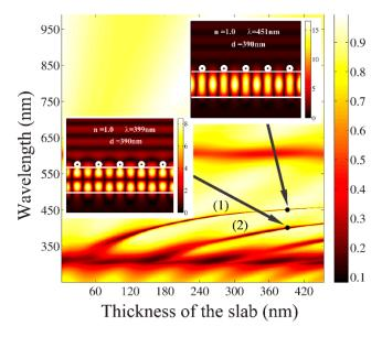
**Figure 7.** Plasmonic grating as refractive index sensor: Contour plots of transmission spectra versus thickness of the slab d at n = 1. Simulated near field distributions of  $|H_z|$  at  $\lambda = 451$  nm and  $\lambda = 399$  nm for a fixed thickness of the slab d = 390 nm are shown as insets.
