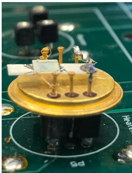
**Figure 1.** Sensor and heater assembly.
