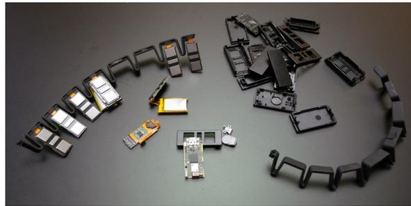
**Figure 2.** Myo armband tear-down [46].
