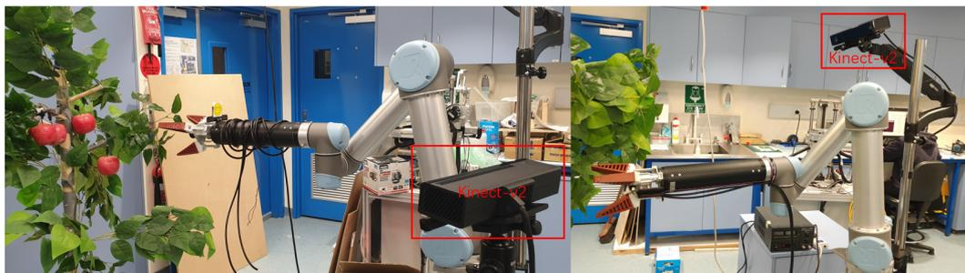
**Figure 1.** The developing apple harvesting robot. The robot comprises a RGB-D camera for vision sensing. A universal robot arm (UR5) is applied as the manipulator.
