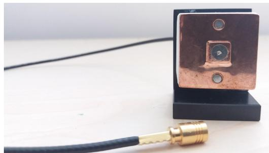
**Figure 6.** Illustration of the design of the copper housing and the printed electrode for the demonstrator setup; the electrical connection was realized through the central hole.
