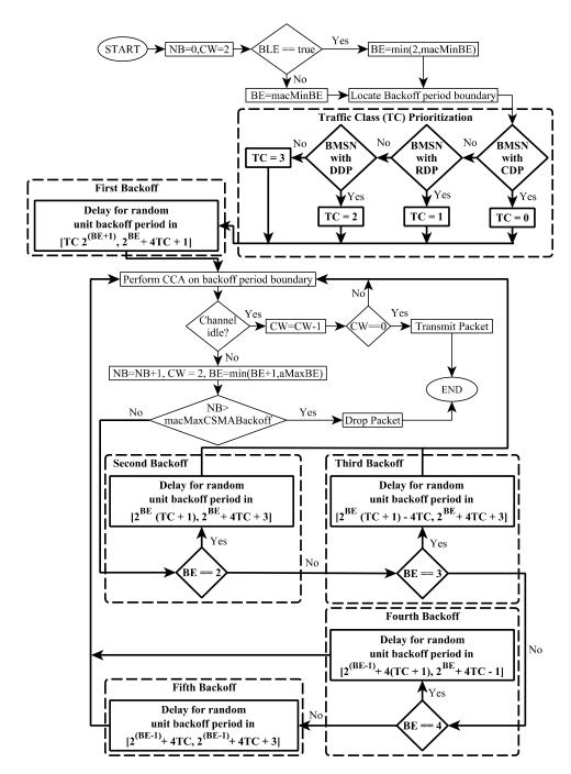
**Figure 1.** Flowchart of Traffic Class Prioritization based Carrier Sense Multiple Access/Collision Avoidance (TCP-CSMA/CA) scheme. The dotted blocks show the contributions made to assign a distinct, minimized, and prioritized backoff period range to each traffic class in every backoff.
