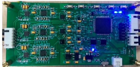
Figure 10. Circuit board of the signal conditioning and processing subsystem.
