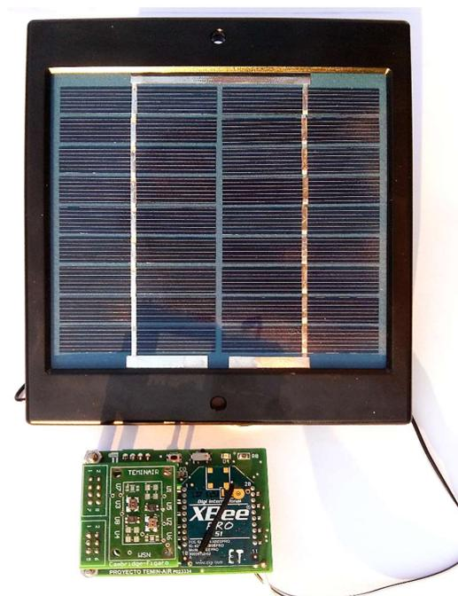
Figure 3. Designed sensor node powered by a solar panel.
