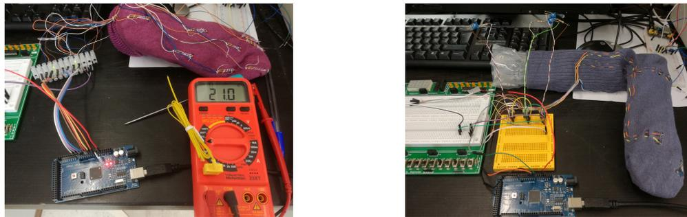
(a) eight NTC sensors and a polymer with a thermocouple (b) PT100 sensors and the auxiliary circuitry
