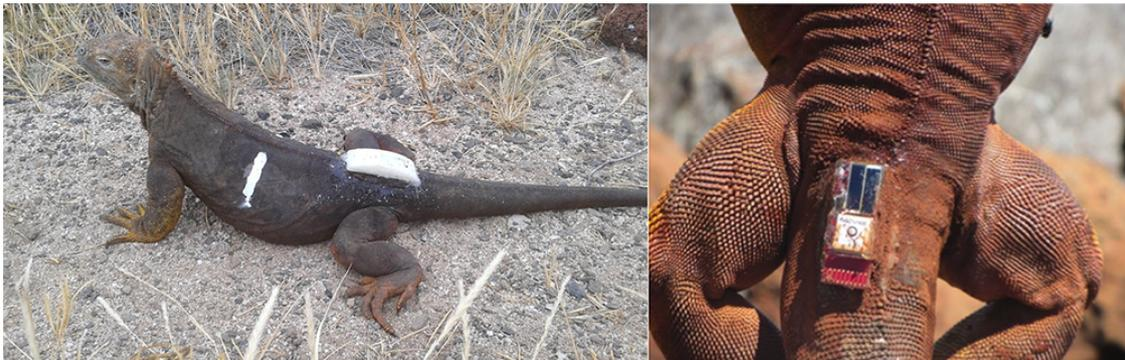
**Figure 5.** On the left, animal with the device glued. On the right, the attachment of the WSN on the iguana back.
