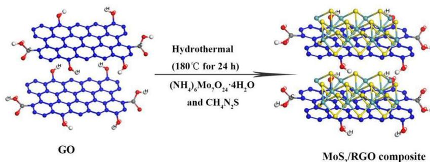
**Figure 1.** Schematic diagram of MoS<sub>2</sub>/RGO composite with reduced graphene oxide (RGO) as template.
