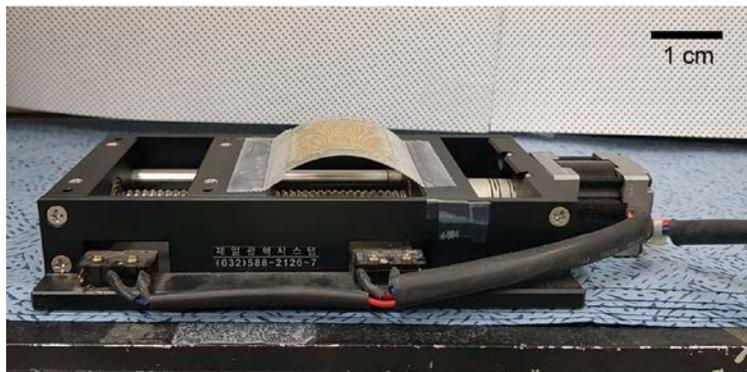
**Supplementary Figure S1.** Photographs of bending machine stage and clamped devices when the energy harvesting signals are measured.
