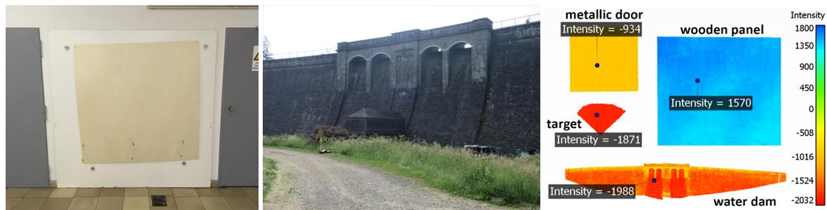
**Figure 1.** Two examples from practice [3]. **Left:** Wooden Panel; **Middle:** water dam; **Right:** Point clouds with intensity values.
