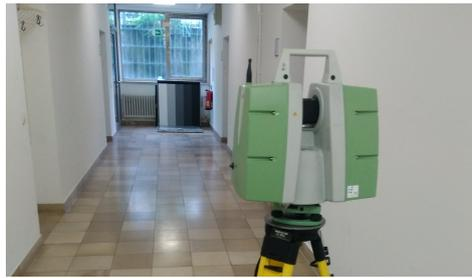
**Figure 4.** Experimental setup to examine reproducibility of intensity values.
