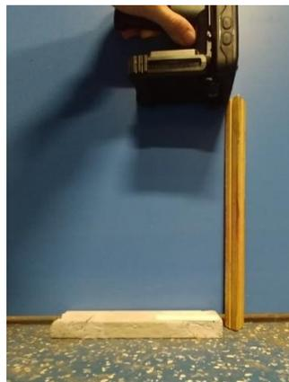
Figure 6. Handheld system crack detection setup.
