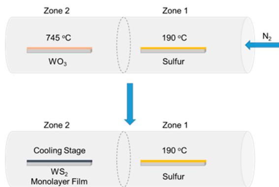
**Figure S3.** Simplified schematic depicting WS<sub>2</sub> fabrication.
