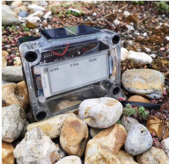
**Figure 3.** Photovoltaic technology provides a staple source of energy for a variety of energy-harvesting systems and is easy to implement as an addition to existing projects. This photo shows polycrystalline photovoltaic technology in use on an embedded sensing platform [36].
