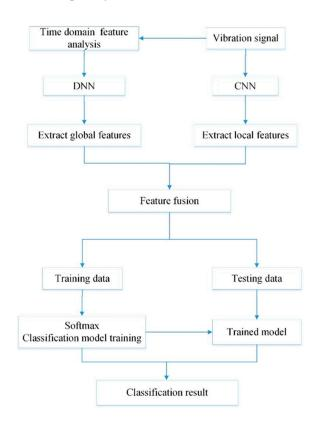
Figure 4. Fault diagnosis process of CNNEPDNN model.
