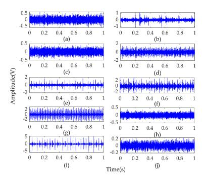
Figure 6. Vibration signals of bearing under 2-hp loads from one sensor. (a–c) are the bearing inner race fault signal under fault size of 7 mils, 14 mils and 21 mils, respectively. (b–d) are the bearing outer race fault under fault size of 7 mils, the 14 mils and 21 mils, respectively. (g–i) are the bearing ball fault under size of 7 mils, 14 mils and 21 mils, respectively. (j) the normal bearing signal.
