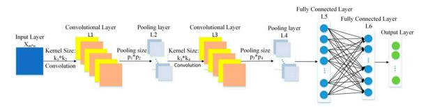
Figure 2. A typical architecture of CNN.
