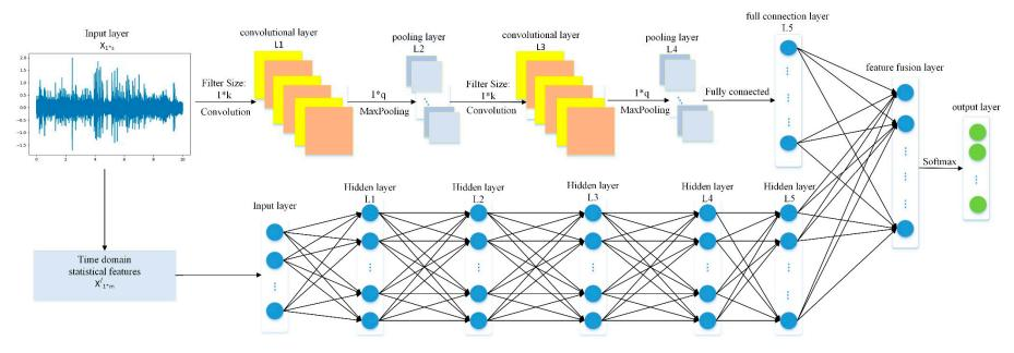
**Figure 3.** Schematic diagram of the proposed model CNNEPDNN.
