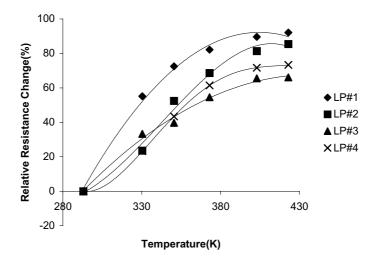
Figure 9. The relative resistance change expressed as a percentage against increasing temperature for the  $In_2O_3/SiO$  samples produced at low pressure.
