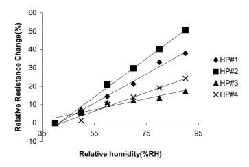
**Figure 13.** Humidity Sensitivity Curves for  $In_2O_3/SiO$ , produced at high vacuum pressure, at  $30^{\circ}C$ .
