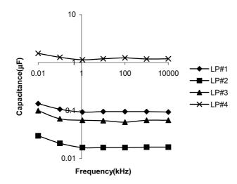
**Figure 5.** The variation of capacitance against frequency for the  $In_2O_3/SiO$  samples produced at low vacuum pressure.
