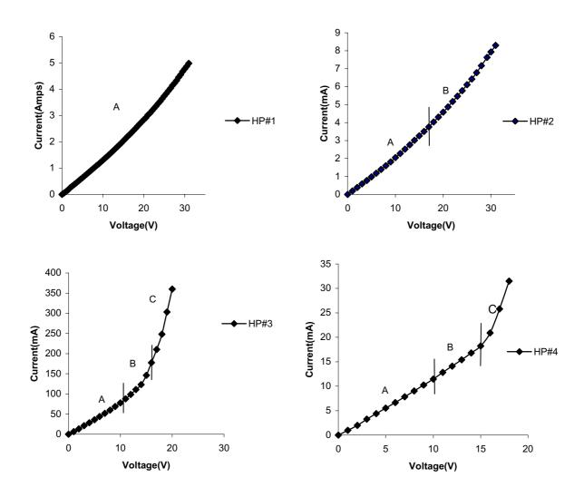
Figure 8. I-V plots for the In<sub>2</sub>O<sub>3</sub>/SiO samples produced at high pressure.
