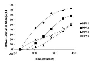
**Figure 10.** The relative resistance change expressed as a percentage against increasing temperature for the  $In_2O_3/SiO$  samples produced at high pressure.
