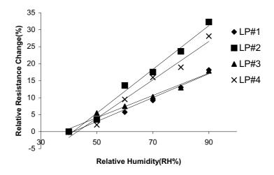
Figure 12. Humidity Sensitivity Curves for In<sub>2</sub>O<sub>3</sub>/SiO at 60°C.
