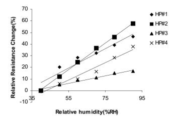
**Figure 14.** Humidity Sensitivity Curves for  $In_2O_3/SiO$ , produced at high vacuum pressure, at  $60^{\circ}C$ .
