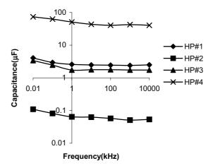
**Figure 6.** The variation of capacitance against frequency for the  $In_2O_3/SiO$  samples produced at high vacuum pressure.
