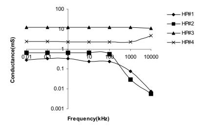
**Figure 4.** The variation of conductance against frequency for the  $In_2O_3/SiO$  samples produced at high vacuum pressure.
