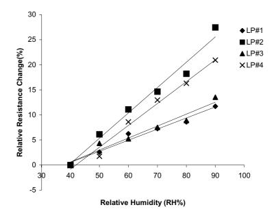
**Figure 11.** Humidity Sensitivity Curves for In<sub>2</sub>O<sub>3</sub>/SiO at 30°C.
