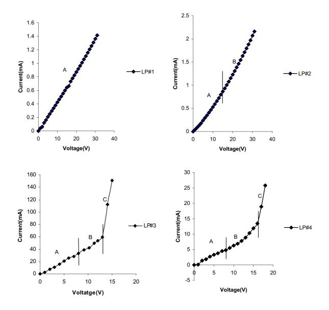
Figure 7. I-V plots for the In<sub>2</sub>O<sub>3</sub>/SiO samples produced at low pressure.
