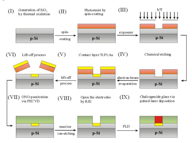
**Figure 1**. Survey on the fabrication steps of the chalcogenide glass-based thin-film sensor array (I: thermal oxidation, II: spin-coating, III: exposure, IV: chemical etching, V: electronbeam evaporation, VI: lift-off process, VII: ONO passivation, VIII: RIE, IX: PLD).
