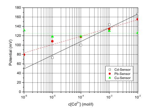
**Figure 7.** Calibration curves of the single sensors of the thin-film sensor array towards Cd2+-ions.
