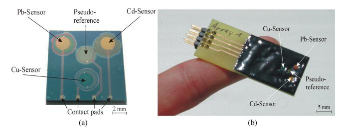
**Figure 4.** (a) Videomicroscopic picture of the thin-film sensor array after the PLD process. The different chalcogenide glasses onto the electrodes are shown. (b) Picture of the complete thin-film sensor array after wire bonding and encapsulation.
