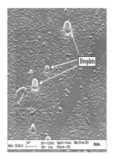
**Figure 5**. SEM micrograph of the surface of the Pb<sup>2+</sup>-selective layer of the thin-film sensor array with chalcogenide glass material system of Pb-Ag-As-I-S.
