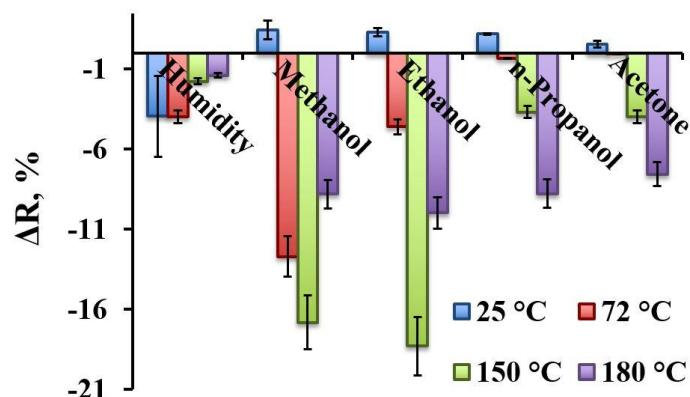
**Figure 8.** The response of TiO<sub>2-x</sub>/TiO<sub>2</sub> (400 °C)-based hetero-structure towards humidity (H<sub>2</sub>O), methanol, ethanol, n-propanol, and acetone at different temperatures (25–180 °C).
