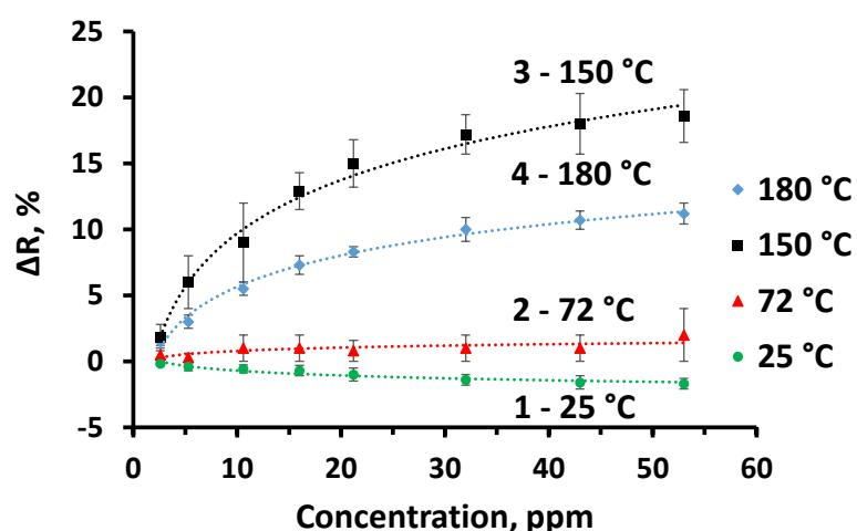
**Figure 9.** The response of TiO<sub>2-x</sub>/TiO<sub>2</sub> (400 °C) hetero-structure towards ethanol, at different temperatures: 25 °C, 72 °C, 150 °C and 180 °C.
