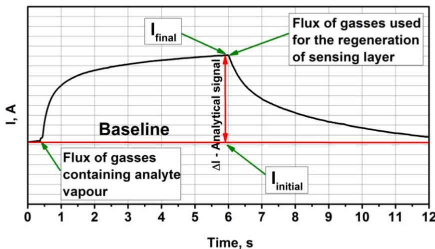
**Figure 2.** Representation of typical analytical signal registered by  $\text{TiO}_{2-x}/\text{TiO}_2$  ( $400\text{ }^\circ\text{C}$ )-based structure. It should be noted that  $\Delta I$ , the duration of signal development and the regeneration of sensor after measurements were different for different gases and different concentrations of those gases.
