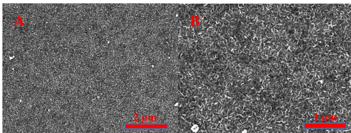
**Figure 3.** Scanning electron microscope (SEM) images of  $TiO_{2-x}/TiO_2$  ( $400^{\circ}C$ )-based hetero-structure at different magnification: (A)—at  $\times 25000$ ; (B)—at  $\times 50000$ .
