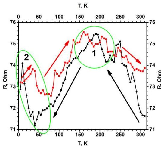
**Figure 7.** Temperature dependence of electrical resistance ( $R(T)$ ) for the  $\text{TiO}_{2-x}/\text{TiO}_2$  ( $400\text{ }^\circ\text{C}$ )-based hetero-structure. Temperature was changed in two ways (indicated by black and red arrows): (i) black cycles shows points measured by cooling down, (ii) red squares shows points by increasing temperature. Measured was performed in vacuum using helium cryostat.
