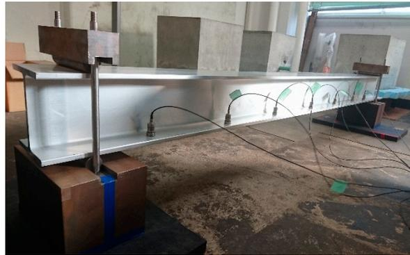
Figure 7. Vibration experiment in this study.
