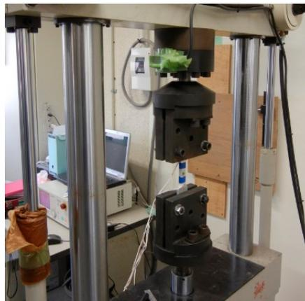
Figure 4. Tensile test of Japanese Industrial Standards No. 5 specimen.
