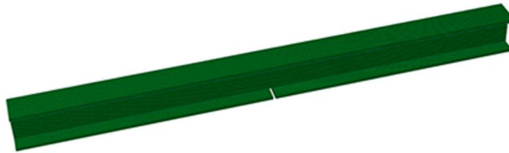
Figure 12. Finite element model of damaged specimen A.
