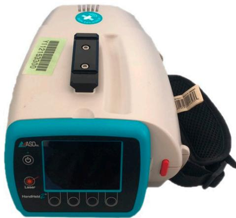
**Figure 3.** ASD FieldSpec HandHeld2 spectrophotometer.
