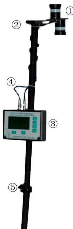
**Figure 1.** Portable three-band instrument of crop-growth monitoring and diagnosis: ① Multi-spectral crop sensor; ② Sensor support; ③ Processor system; ④ Shielded cable; ⑤ Level.
