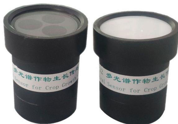
**Figure 2.** Multispectral sensor.
