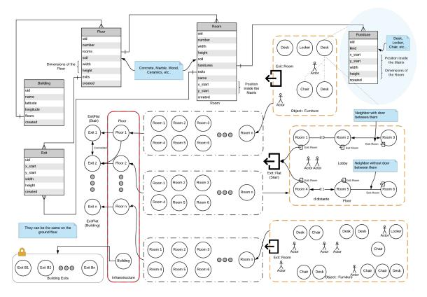
**Figure A1.** Model of the internal structure building, stored in a graph with their respective relationships and content nodes.
