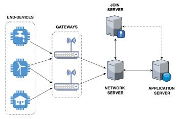
Figure 1. Architecture of a LoRaWAN Network.
