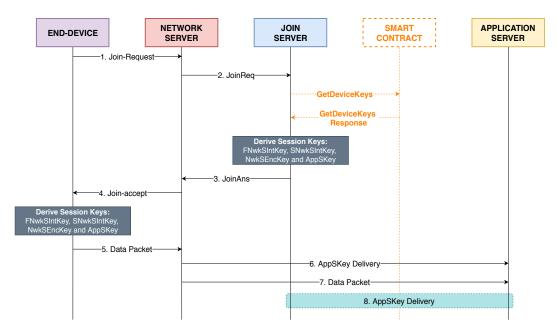
Figure 4. End-device authentication and data transmission in the proposed architecture.
