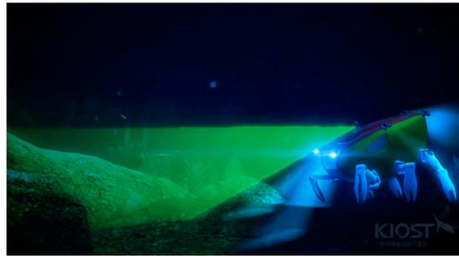
Figure 10. Tilt angle adjustment to the sector-scanning sonar concept for the CR200 [25].
