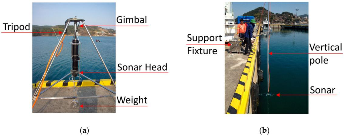
**Figure 1.** General sector-scanning sonar image acquisition methods: (a) Horizontal image acquired by tripod deployment; (b) Vertical image acquired by pole-mount deployment.
